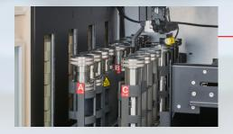
Use nitrogen and vacuum at the same time to expedite evaporation. Gentle heating may also be applied if desired. The vacuum is set at a low level so semi-volatile compounds will not be lost.
