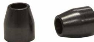
Two types of Vespel/graphite are commonly used, one with 40% graphite and one with 15% graphite. They are ideal for GC/MS interface applications because they are non-porous to oxygen. The inclusion of graphite increases high-temperature tolerance and reduces sticking and shrinkage.
