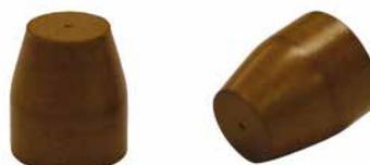
Vespel GC ferrules are excellent for creating seals on metal or glass and have long lifetimes. 100% Vespel is essentially non-porous to oxygen so it is ideal for GC/MS interface use, where air permeation can raise the background signal and contribute to phase degradation. They also work best in connections that are isothermal or insulated from oven temperature changes.
